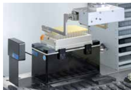
Robotic Gripper Arm with eccentric grippers loading a 2-D bar code reader
