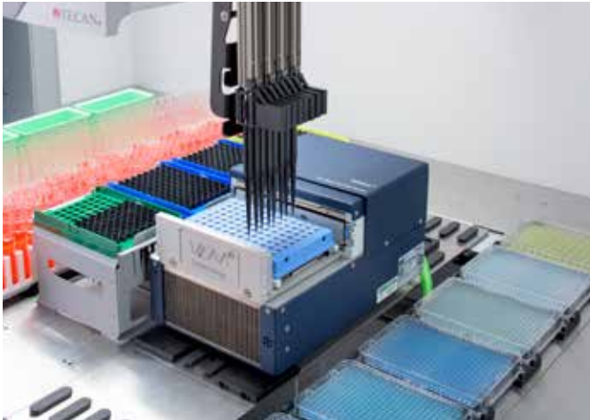
Pipetting directly into thermocycler
