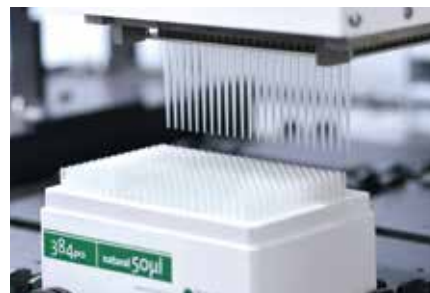
Multiple Channel Arm 384 picking up one column of 50µl tips
