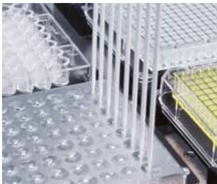
Piercing with fixed washable tips and liquid displacement Flexible Channel Arm
