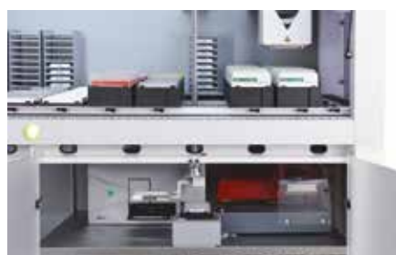
Below deck integration of a centrifuge
