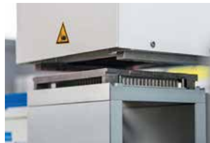
Multiple Channel Arm 384 picking up disposable tip adapter
