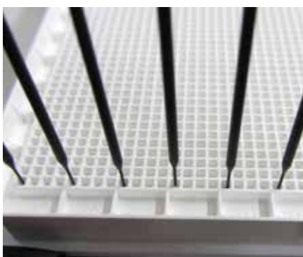
Flexible channel arm with Te-PS tips pipetting into 1,536 microplate
